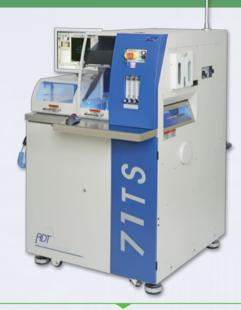
The Tilting Spindle dicing system is designed to meet the needs of Optoelectronic component manufacturers by providing both perpendicular cuts and 8° angular cuts needed to suppress backreflection in fiber optic components.
