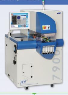
ADT 7900 series has two facing spindles that can simultaneously dice wafers or packages at high throughput. ADT 7900 series is a high accuracy system that can dice product at high performances and low cost of operation.
