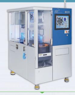
ADT 8020 Dicing system has two facing spindles that can simultaneously dice wafers at high throughput. ADT 8020 is a high accuracy system that can dice product up to 8" in diameter, at high performances and low cost of operation.
