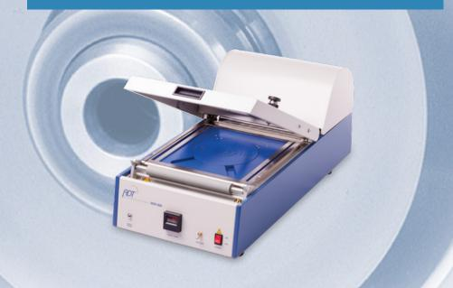
Designed for manual mounting of workpieces on tapes. Supporting various types of dicing tapes and standard frames. Can be customized for multiple substrates (multi-panel) and irregular frames.
