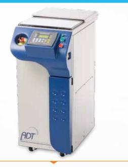
Designed for after-dicing workpiece cleaning and drying. Equipped with a spinning chuck table and a rotating washing/drying arm. The arm can be configured with an atomizing cleaning nozzle or a high pressure nozzle to cope with a wide range of cleanliness requirements.
