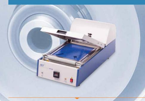
Designed for manual mounting of workpieces on tapes. Supporting various types of dicing tapes and standard frames. Can be customized for multiple substrates (multi-panel) and irregular frames.
